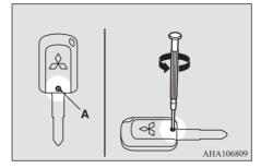
3. With the MITSUBISHI mark facing you, insert the cloth-covered tip of a straight blade (or minus) screwdriver into the notch in the remote control switch case and use it to open the case.
