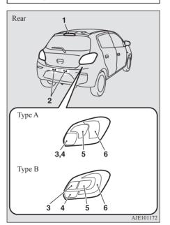
Type A: Bulb type stop and tail lamps
