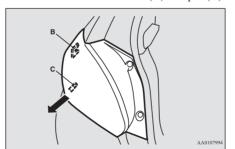
4. Turn the socket anticlockwise to remove
