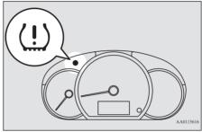
When the ignition switch is turned to the "ON" position, the tyre pressure monitoring system warning lamp normally illuminates and goes off a few seconds later.
