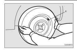
7. Temporarily tighten the wheel nuts by hand until the tapered parts of the wheel nuts make light contact with the seats of the wheel holes and the wheel is not loose.
