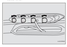
5. Pull the bulb out of the socket.
