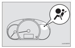
There is a supplemental restraint system ("SRS") warning lamp on the instrument panel. The system checks itself every time the ignition switch is turned to the "ON" position or the operation mode is put in ON. The SRS warning lamp will come on for several sec-
