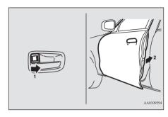
Set the inside lock knob (1) to the locked position, and close the door (2).
