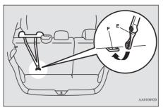
Push and pull the child restraint system in all directions to be sure it is firmly secured. Installing a child restraint system to a 3-point type seat belt (with emergency locking mechanism) or a lap belt
