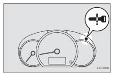
When the operation mode is in any mode other than OFF, if you try to lock the doors and tailgate by pressing the driver's door lock/unlock switch, or the tailgate lock/unlock switch, a warning lamp will blink and the outer buzzer will sounds for approximately 3 seconds and you cannot lock the doors and tailgate.
