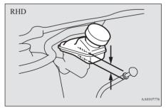
The fluid level is monitored by a float. When the fluid level falls below the "MIN" mark, the brake fluid warning lamp lights up.
