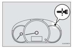
If the operation mode is in OFF and the driver's door is opened with the keyless operation key in the key slot, the warning lamp will blink and the outer buzzer sounds for approximately 3 seconds and the inner buzzer sounds for approximately 1 minute to remind you to remove the key.
